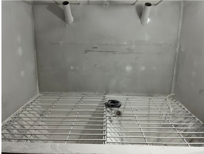
Picture 3: IP6X test view of models BLU-TITAN-R6
