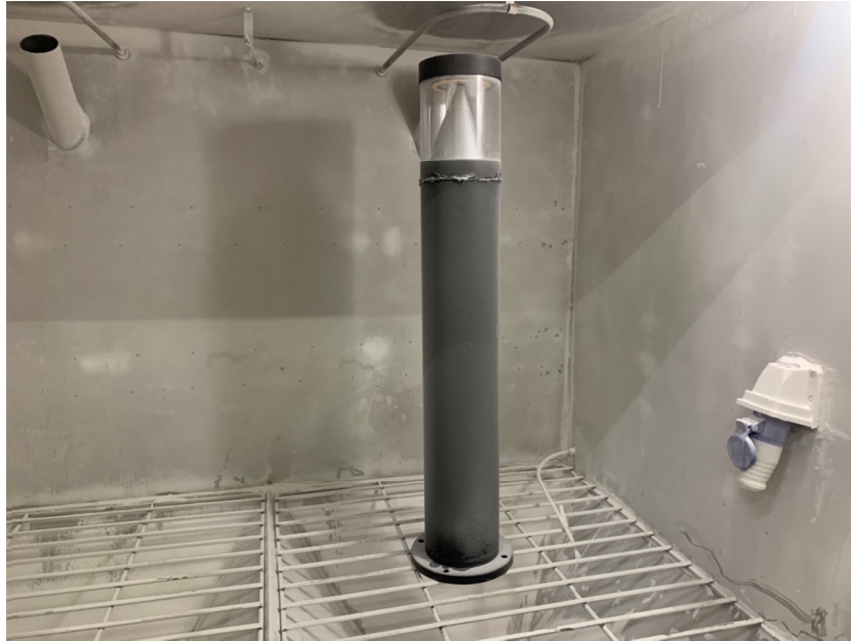
Picture 1: IP6X test of model BLU-STKC-15W-827-B
