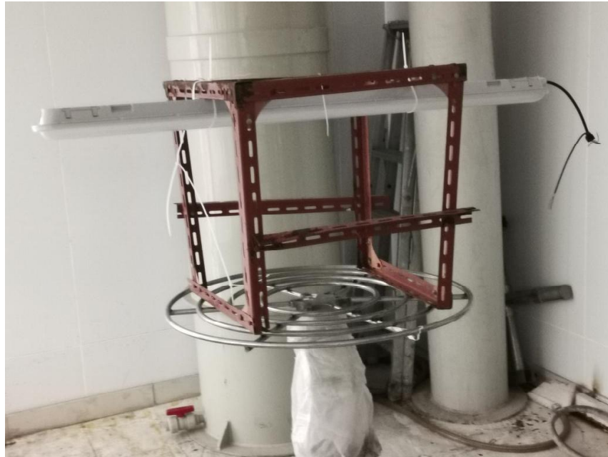
Picture 2: IPX5 test of model BLU-ECO-120-40W
