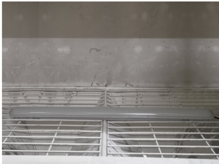
Picture 1: IP6X test of model BLU-ECO-120-40W
