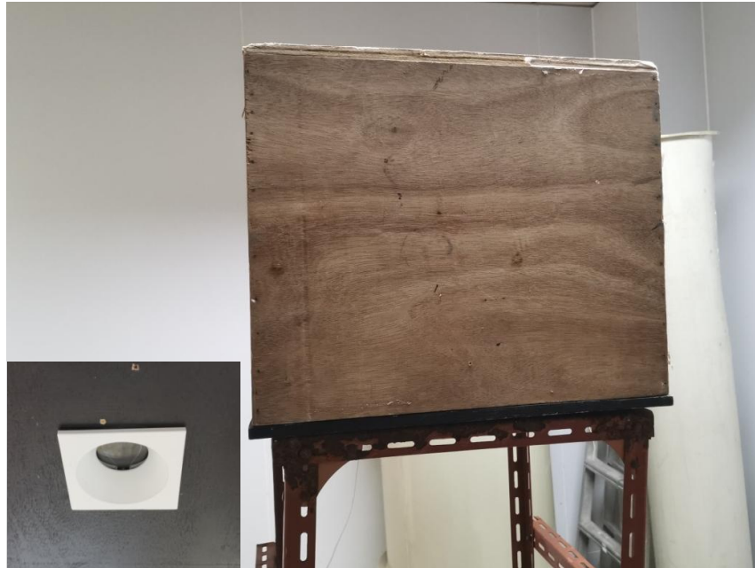
Picture 2: IPX5 test of model BLU-SPLASH-8SF-W
