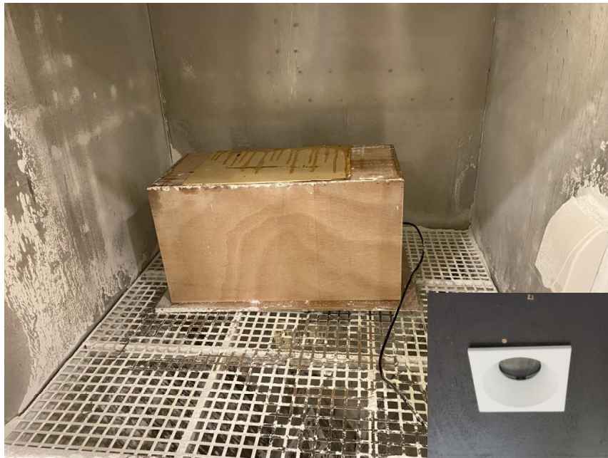
Picture 1: IP6X test of model BLU-SPLASH-8SF-W
