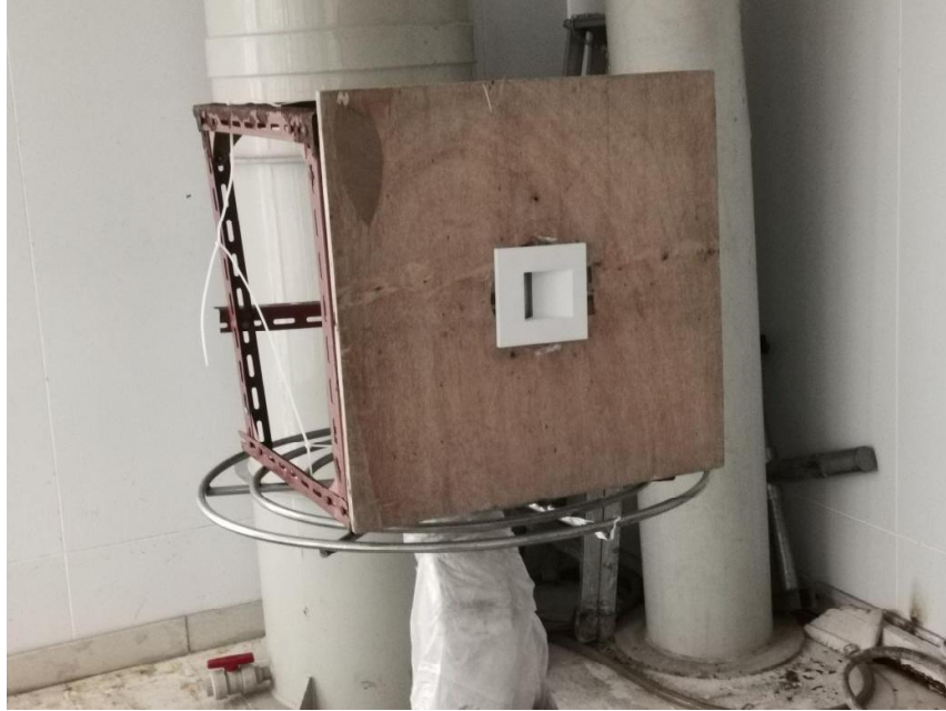
Picture 2: IPX5 test of model BLU-STEPZ-S10-10W
