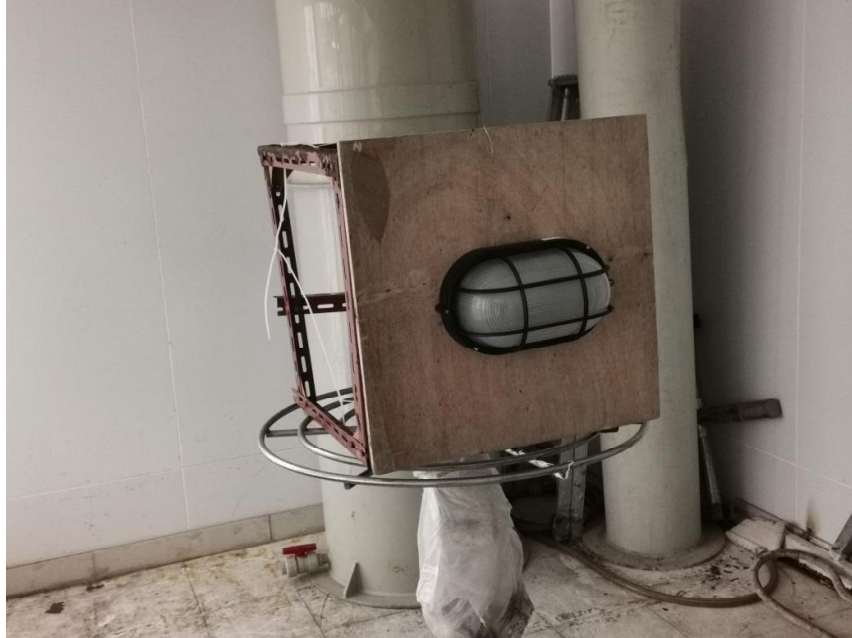
Picture 2: IPX5 test of model BLU-BULKZ-OVG-10W
