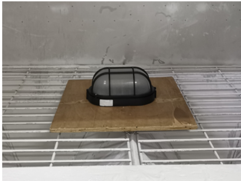
Picture 1: IP6X test of model BLU-BULKZ-OVG-10W
