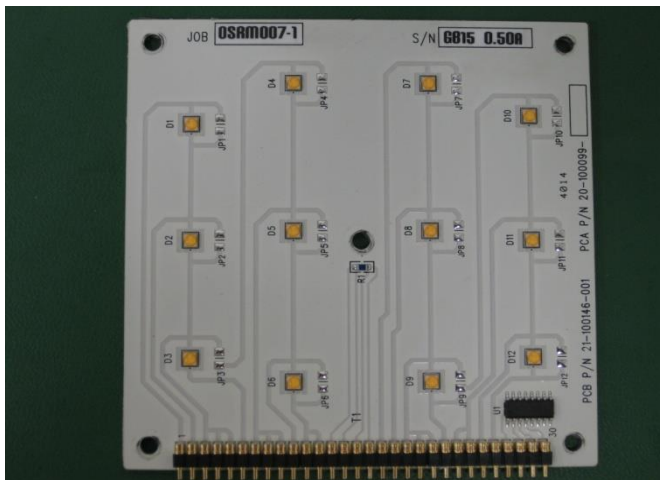
Fig. 1 Load board with 12 samples. Absorption correction measurements are made for each load board measurement.
