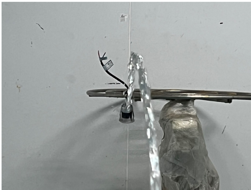
Picture 2: IPX5 test view of model BLU-STEPZ-R5
