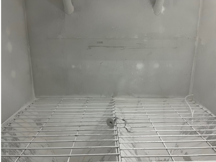
Picture 3: IP6X test view of model BLU-STEPZ-R5
