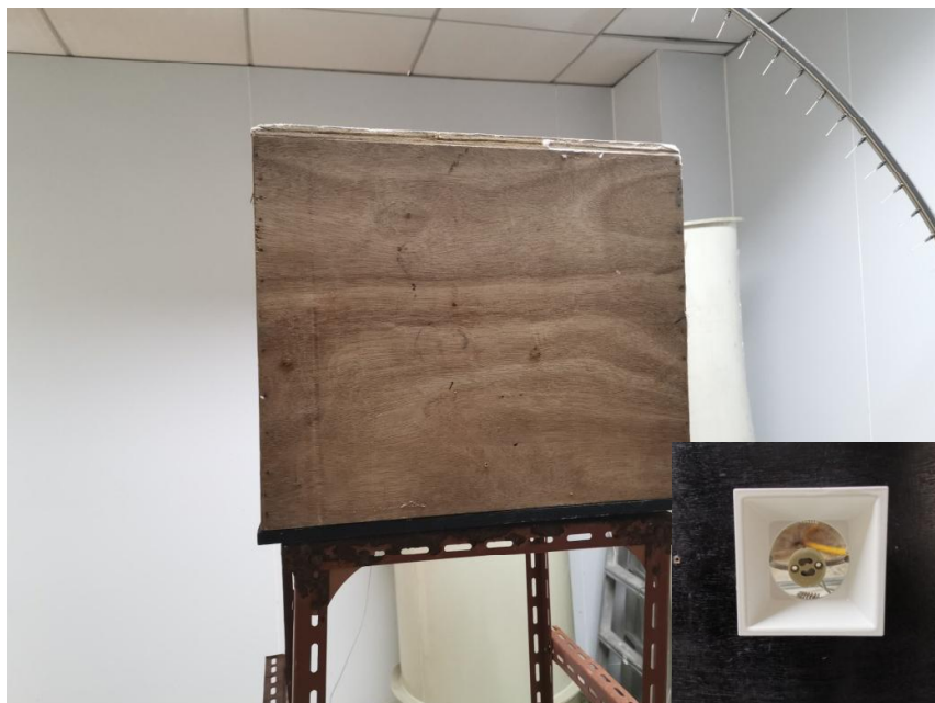
Picture 2: IPX4 test of model BLU-AIM-8SA-W
