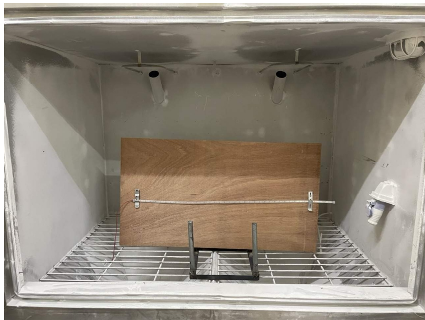
Picture 5: IP6X test of model BLU-FLEXI-7.2W-927-IP67
