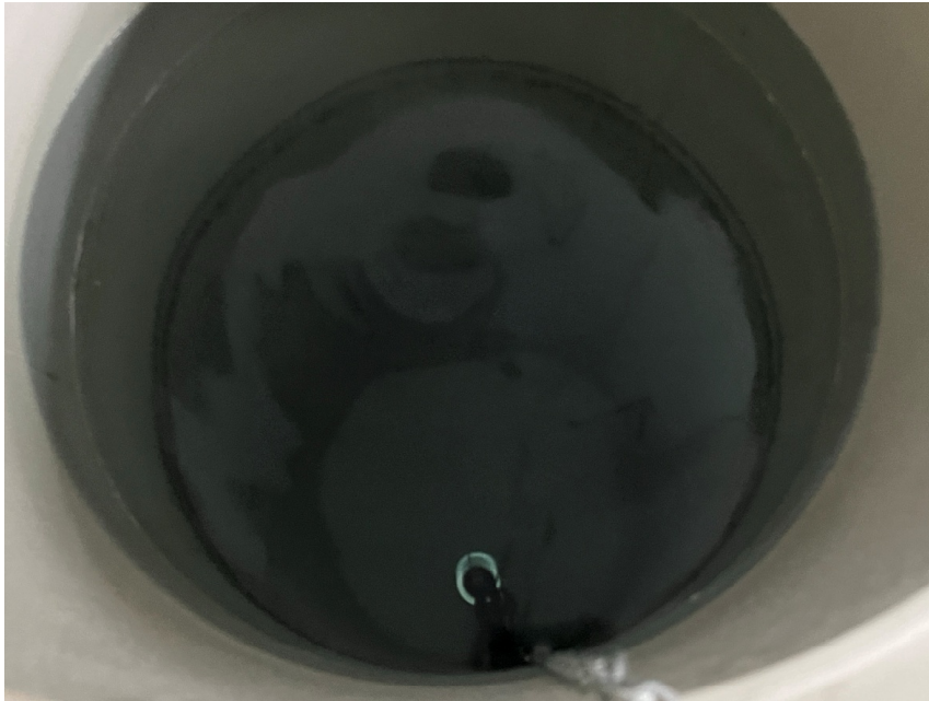
Picture 3: IPX7 test view of models BLU-ROOTZ-L100 and BLU-ROOTZ-L50
